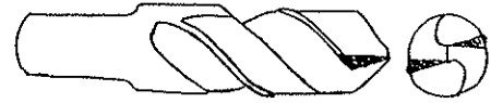
TO "DERAKE" A DRILL BIT, GRIND AWAY THE SHADED PORTION SO THAT THE CUTTING EDGE IS PARALLEL TO THE SHAFT INSTEAD OF SLIGHTLY OBLIQUE
